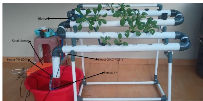
Fig. 5 Hardware Placement on Hydroponic NFT System
