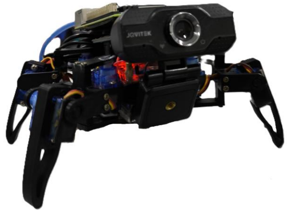
Figure 4. The assembled ArachnoSAR prototype: four 2-DOF legs driven by eight SG90 servos, a front-mounted Jovitech CM07 webcam, and on-board control electronics
